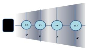
Testing was conducted in compliance with ANSI EOS/ESD S3.1-1991 of the ESD Association. Decay times in seconds. Distance in feet.
