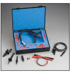
**Model 2187-4 Test Lead Kit:** Includes an input cable with banana terminations, banana extensions, sprung-hook clips, alligator clips, needle probes, and spade lugs to connect the Model 2182A to virtually any DUT. The kit is also used to connect the Model 2182A directly to the Model 622X guard to improve response time for pulsed measurements or to reduce errors when measuring high impedance devices.
