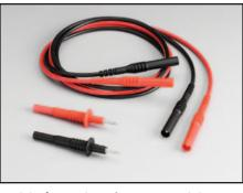
**Model 8605 High Performance Modular Test Leads:** Highest quality lead with silicone insulation, and removable test probes. Rated to 1500V. UL listed. **Length:** 1m (3.3 ft).
