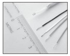
**Model 8681 Low Cost RTD:** This inexpensive RTD has small size (0.09 in  $\times$  0.09 in) and fast thermal response time. 100 $\Omega$ , 0.385%/°C element. Meets or exceeds DIN 43760-1980-A, IEC 751:1983-A, BS1904: 1984-A, and JIS C1604-1981-0.2. Can be used with Model 8680 RTD Input Probe Adapter. Measures from  $-200^{\circ}$  to  $+600^{\circ}$ C.
