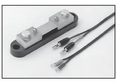
**Model 1651 50 Ampere Shunt:** External  $0.001\Omega \pm 1\%$ , 4-terminal shunt; extends current measuring capability of Keithley DMMs to 50A.
