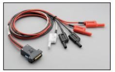
**Model 3706-BAN:** 1.4m (4.6 ft) banana test leads/adapter cable for Model 3706 mainframe with high performance multimeter option. Provides direct connection to high performance multimeter utilizing rear panel backplane connector. Safety banana connections to HI, LO, Sense HI, Sense LO, and AMP.
