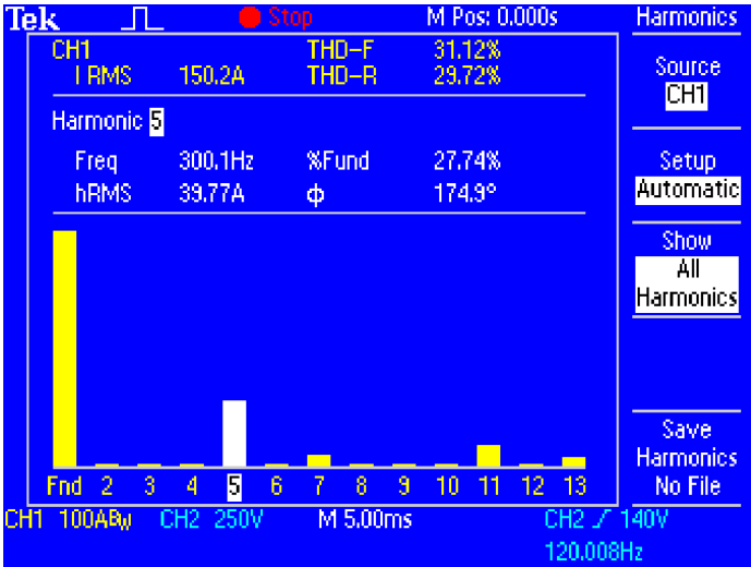
Conduct harmonic distortion measurements with TPS2PWR1 software.
