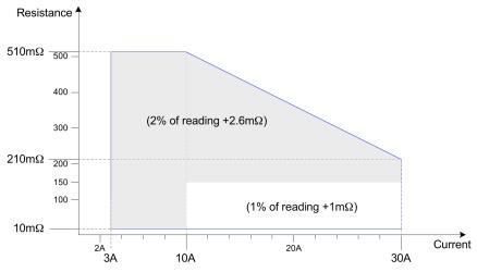
**Output Current:** Range: 3.00A to 30A AC Resolution: 0.01A, 3-30A
