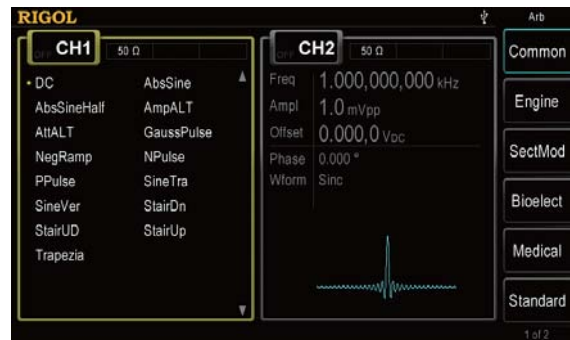
Arbitrary waveform function and built-in 150 waveforms
