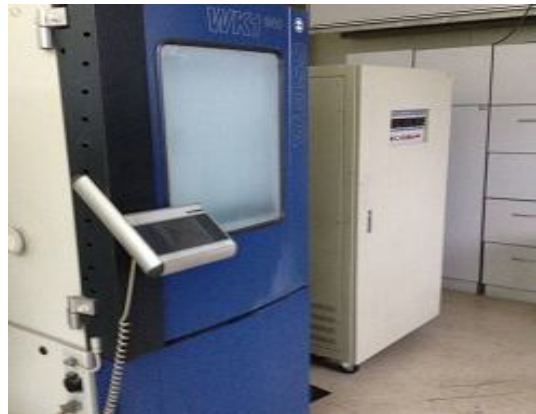
b. Temperature/Thermal Chamber Test
