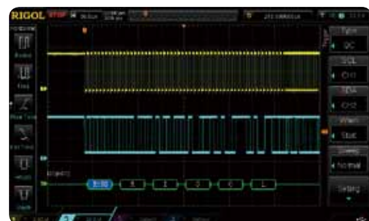
Optional Serial Bus Triggering and Decoding functions(RS232,I2C,SPI)
