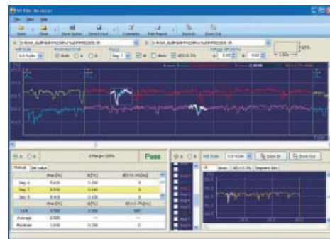
▲Example of test results in the case of manual switching
