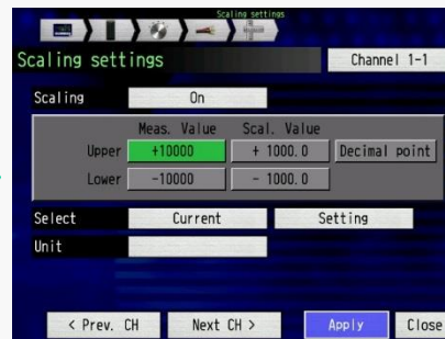
Select the "Upper" and "Lower" values for the "Meas. Value". (Measured Value)
