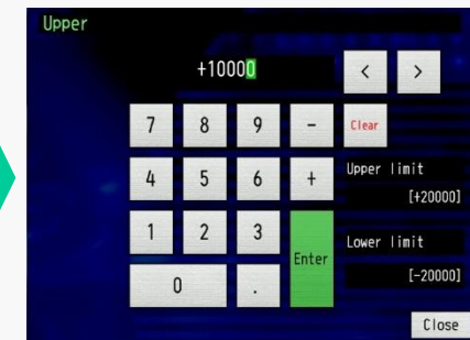
Enter the value. If set value is out of the limit, measuring range will need to be changed.
