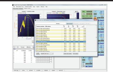
Import module data from embedded Sandia database and create I-V Curve
