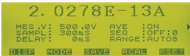
Data display with 0.1 fA resolution (10 pA range).
