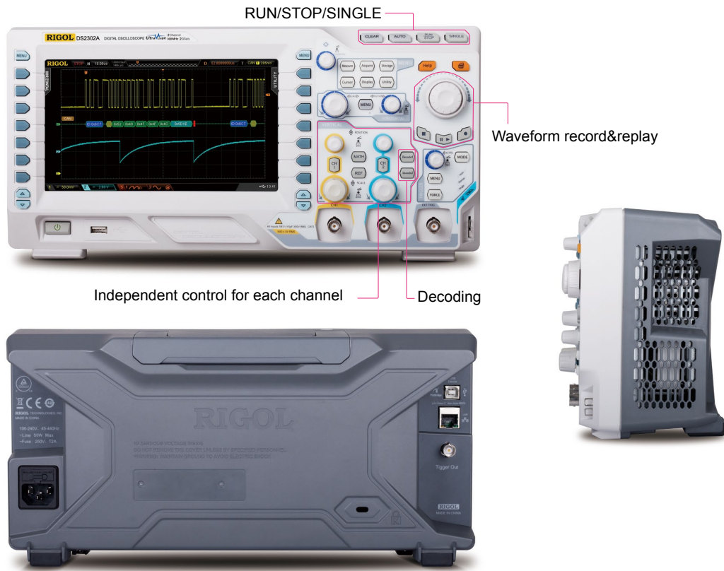
Product Dimensions: Width X Height X Depth=361.6 mm×179.6 mm×130.8 mm Weight: 3.9 kg ± 0.2 kg(Without Package)
