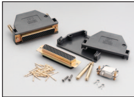
Model 3791-KIT78-R: 78-pin female D-sub connector kit that contains two female D-sub connectors and 156 solder-cup contacts. Use for assembly of custom cable and harnesses compatible with Series 3700 plug-in cards.
