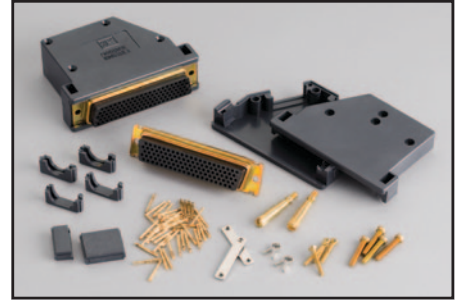
Model 3792-KIT104-R/F: 104-pin female D-sub connector kit that contains two female D-sub connectors with housings and 208 solder-cup contacts. Use for assembly of custom cables, harnesses, and DUT interface compatible with Series 3700 plug-in cards.
