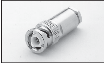
CS-631: 3-slot male triax cable mount connector for use with SC-22 cable. Mates to Models 237, 486, 487, 7072, and 8006. For use with: 4200-SCS, SC-22 cable
