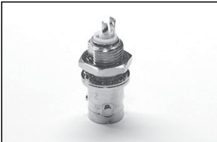
CS-630: 3-lug female triax bulkhead connector for soldered connection. Mates with CS-631. For use with: Fixtures, 6487, 6517A, 6517B
