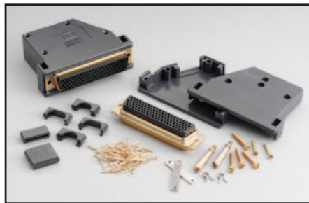
Model 3791-KIT104-R: 104-pin male D-sub connector kit that contains two male D-sub connectors with housings and 208 solder-cup contacts. Use for assembly of custom cable and harnesses compatible with Series 3700 plug-in cards.
