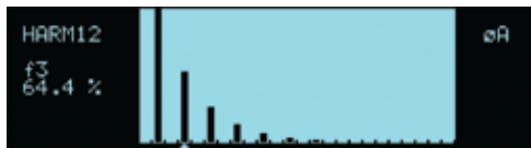
Harmonic waveform, Fund., 3rd, 5th, 7th, 9th, 11th and 13th.
