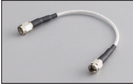
CA-405B: 15cm (6 in) RG188 coax cable terminated with an SMA male plug on each end, 50 \Omega impedance.
