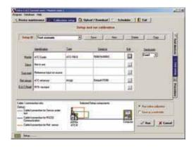
The JOFRACAL calibration software supports automatic calibration for all JOFRA dry-block calibrators equipped with an RS232 serial data interface including the JOFRA DTI050 digital thermometer, the JOFRA DTI-1000 digital thermometer and the JOFRA ASM Multi-scanner.
