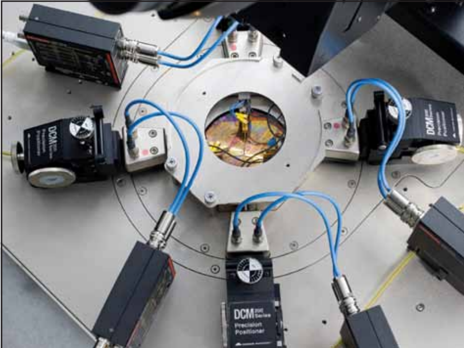
This top-down view of a Cascade Microtech analytical probe station illustrates best practices for interconnecting the Model 4225-RPM Remote Amplifier/Switch to the prober using the blue Multi-Measurement Performance cables.
