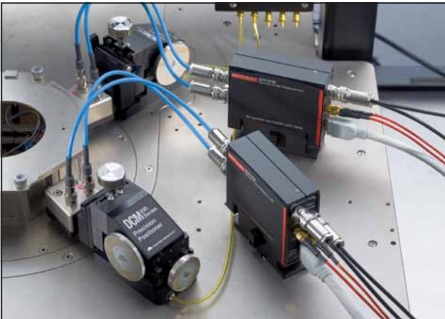
This close-up of two Model 4225-RPMs highlights the DC SMU, C-V, and ultra-fast I-V cable connections.
