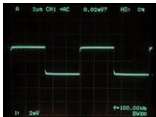
Input: 100 kHz square wave 400 mAp-p (Oscilloscope bandwidth 100 MHz)
