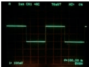
Input: 100 Hz square wave 20 Ap-p (Oscilloscope bandwidth 100 MHz)
